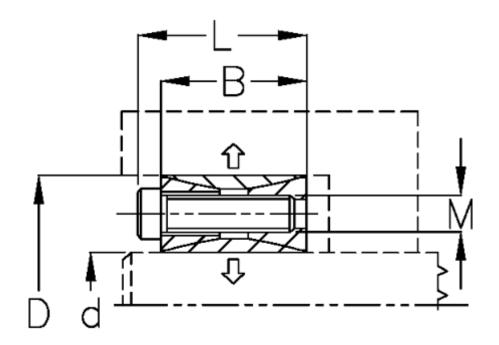
$\begin{array}{lll} \text{B mm} & = 20 \\ \text{d H8 mm} & = 30 \\ \text{D mm} & = 55 \\ \text{Fit tolerance} & = \text{Aksel k11-h11, Nav N11-H11} \\ \text{F kN torque} & = 20.6 \\ \text{L mm} & = 26 \\ \text{M mm} & = M6 \\ \text{P N/mm2 surface pressure on shaft/hub} = 34 \\ \end{array}$
